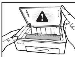
2. Lift the ribbon door. The printing head needs to be heat up to perform the intended functions of the product properly.
