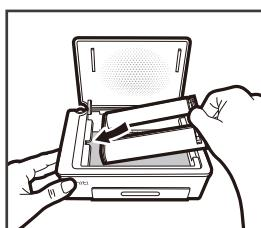
3. Follow the arrow direction marked on the Ink Ribbon and inside the printer, and then slide the Ink Ribbon into the empty compartment.
