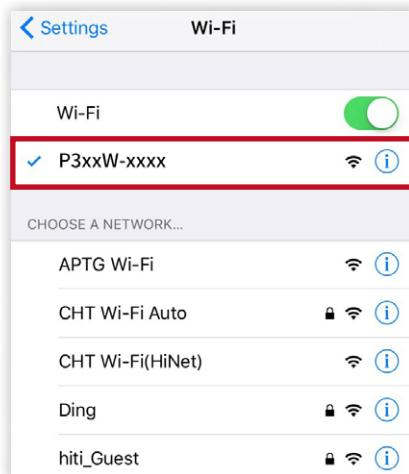
Turn on the printer and go to the WiFi Setting page on your mobile device to find “P3xxW-xxxx.” Tap on the device name to connect to the printer.
