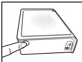
1. Press on the Ribbon Door Switch to lift open Ribbon Door.
